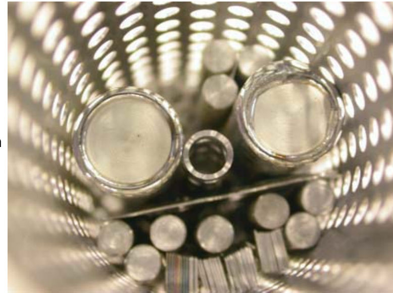
Vanadium specimens in basket to be immersed in molten lithium during irradiation
