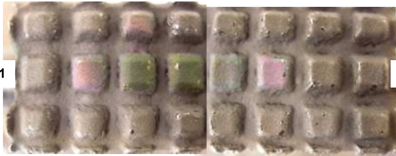
Beryllium near net shaped plasma spray on pre-castellated copper heat sink
