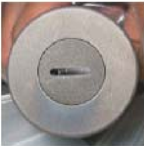
Slotted DiMES experiment in DIII-D showed soft layer of Carbon deposited in the slot with a preliminary atomic C/Deuterium ratio of 0.2-0.6
