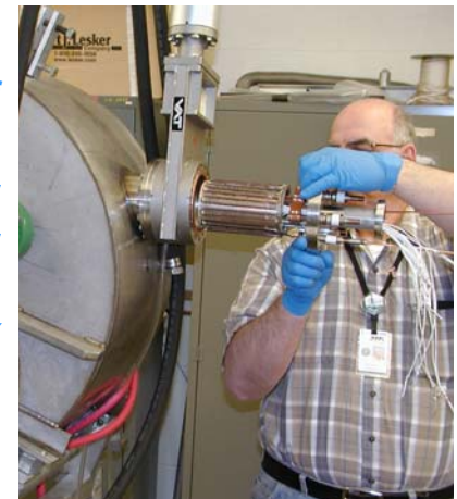
Testing of Lithium evaporator systems for producing thin Li films in NSTX
